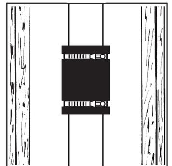
Support pipe and test\* for leaks before concealing joint.
