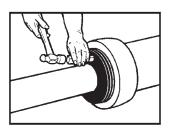
Insert Donut and spigot assembly into the opening. Drive Donut with hammer and wedge until fully seated.
