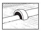
Test joint to engineer's specifications. Pressure test before backfilling or concealing. Bed and backfill properly.
